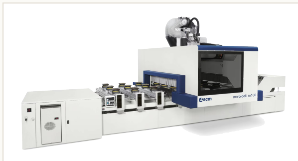
AUTOMATED DOOR LINE · KDT Squaring, boring, edging and finishing in one continuous, automated flow.
